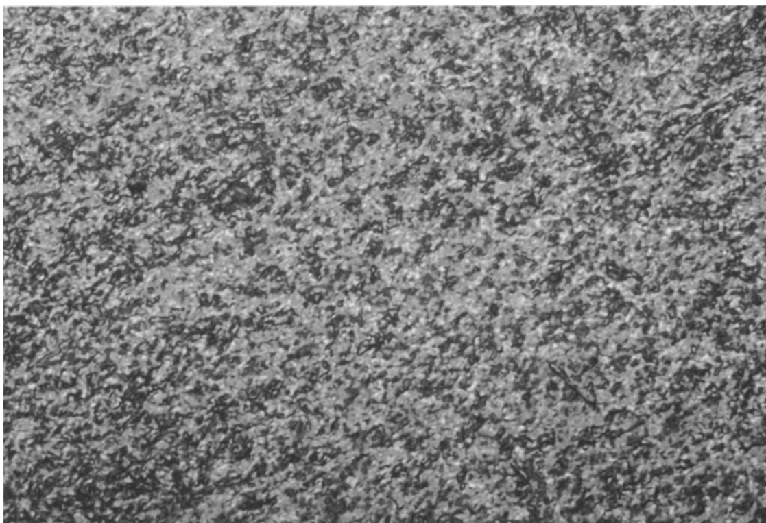
Fig. 1b. Nematic threaded texture of PDCE at 84°C (crossed polarizers). \times 400 .
