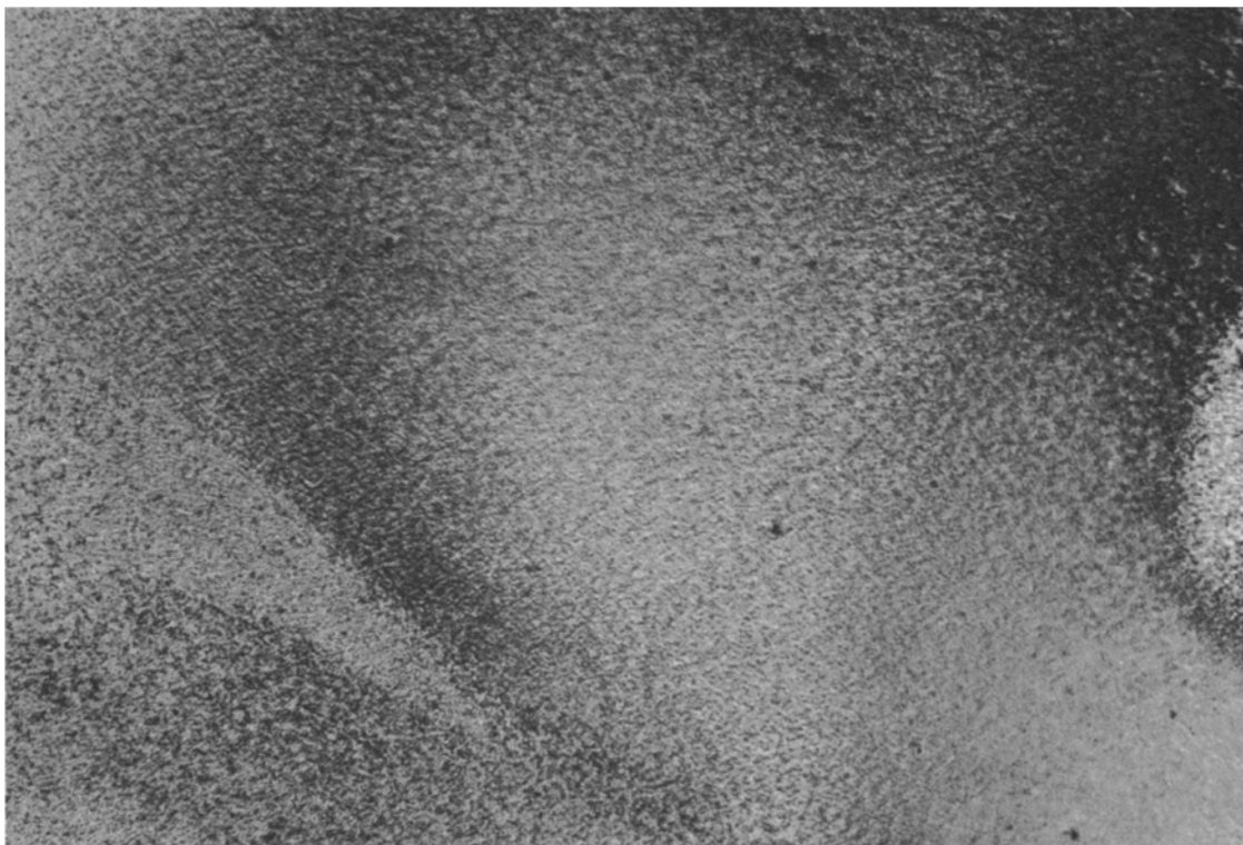
Fig. 1a. Nematic texture of PDCE at 84°C (crossed polarizers). \times 100 .
